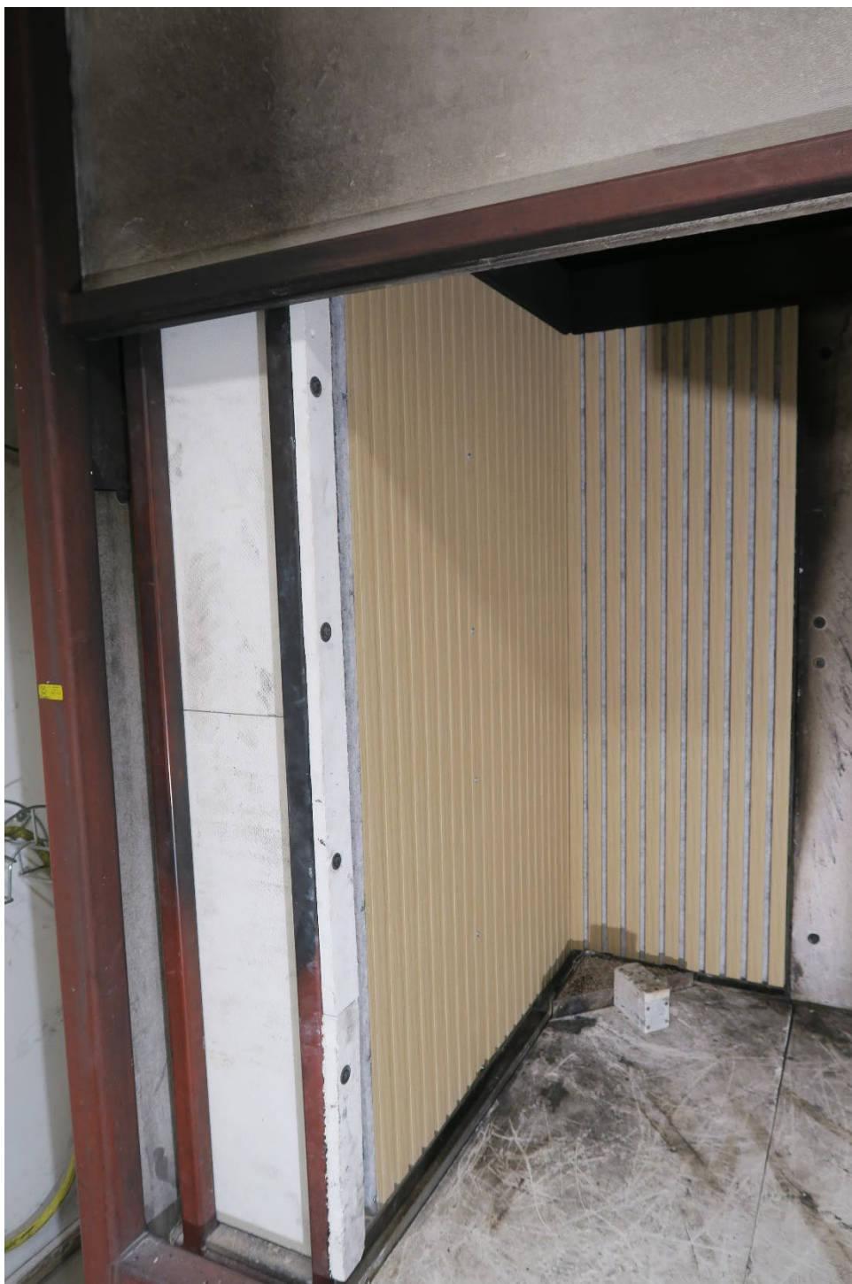
Photo no 2 Prior to test “Acoustic Panel”
